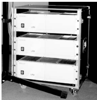
Fig. 13.11. Three 16-channel audio amplifiers for the array in Fig. 13.10 mounted in a 19 inch rack.
