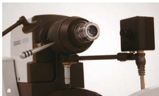
Fig. 2.21 Confocal noncontact fluorescence laser-scanning microscopes [Rostock Cornea Module (RCM)–Heidelberg Retina Angiograph (HRA) II]. a RCM (noncontact) adapted for the HRA II. b Noncontact micrograph of sodium fluorescein-stained epithelium after laser-assisted in situ keratomileusis (LASIK)
