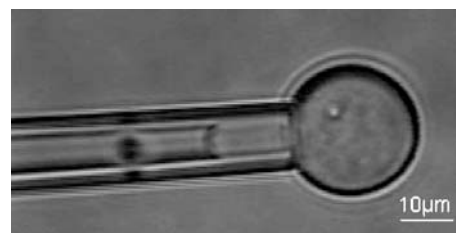
Fig. 5 Micropipette aspiration of a sol-filled vesicle held by micropipette suction ( 10^4 Pa)
