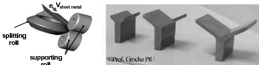
Fig. 1. Process Principle and produced simple geometry
