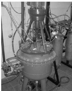
Fig. 2. The stirred tank reactor with heating-cooling jacket
