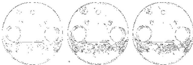
Fig. 9. Results of grouping of image feature-carriers by using the modified Hough transformation for l\_gap = 1, l\_joint = 10 (left); l\_gap = 1, l\_joint = 5 (middle); l\_gap = 2, l\_joint = 10 (right)
