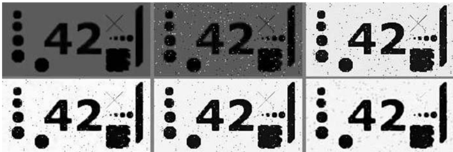
Fig. 2. Clustering results of an image corrupted with a salt & pepper noise. Shown left-to-right and top-to-bottom are: image, corrupted image, clustering results for FCM, FAVG, FMED and FMYR
