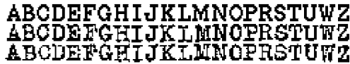
Fig. 6. Upper case: manual designed model letters (upper row) and real typewriter restored prints subjectively arranged in two visual qualities – rather good (middle row) and rather poor (lower row)
