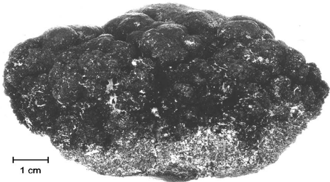
Fig. 11.9 Hamburger-shaped nodule from the Clarion-Clipperton F.Z. region displaying a smooth surface texture on the upper surface and a rough surface texture on the underside (l [D] b s ). Sample collected at Stn 321 GBH, R.V Sonne cruise SO-25 (7°57.30'N, 143°28.92'W, 5153 m). Photograph courtesy of U. von Stackelberg, BGR.
