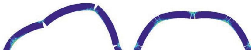
Fig. 1. (a) Four and (b) five hinge collapse mechanisms, for quarter span and middle span loading, respectively.
