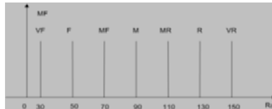
Fig 6. Membership functions plot for output variable Surface Roughness
