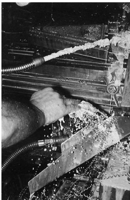
Fig. 11. A machine tool operator deflecting soluble oil to check the machine setting
