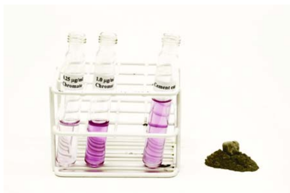
Fig. 1.2. Detection of chromate in cement. A few drops of the reagents were added to the reference solutions and to the cement extract. The red-violet color of the extract indicates the presence of chromate in the investigated cement
