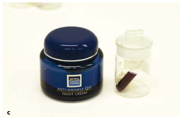
Fig. 1.4a–c. Detection of formaldehyde with the chromotropic acid method. Violet color of the reagent indicates the presence of formaldehyde. a One blank and two standard solutions of formaldehyde. b Products to be analyzed. c A leave-on product containing formaldehyde
