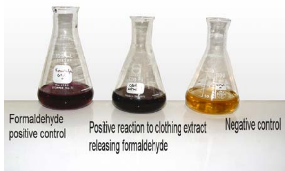
Fig. 21. Positive reaction with chromotropic acid method, showing liberation of formaldehyde by textile resins (formaldehyde solution on the left as a positive control, negative control on the right)
