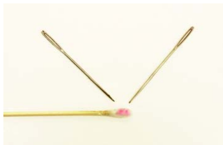
Fig. 1.1. Detection of nickel ions released from sewing needles. A few drops each of dimethylglyoxime 1% in ethanol and ammonia 10% in water were applied to the cotton-tipped applicator, which was rubbed against the needles. The pink-red color of the cotton indicates the presence of nickel ions
