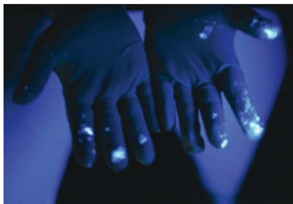
Fig. 2.1. Contamination of protective gloves with dental acrylates, visualized by the fluorescence tracer technique (courtesy of A. Boman).
