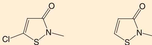
Scheme 5. Methylchloroisothiazolinone and methylisothiazolinone
