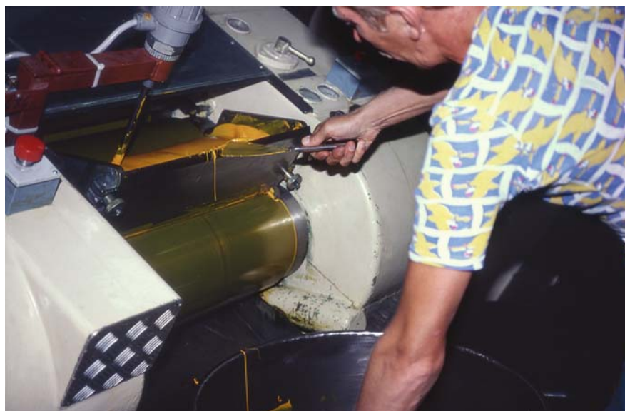
Fig. 1.3. UV-curable acrylic inks mixed with color pigments. Protective gloves are highly recommended
