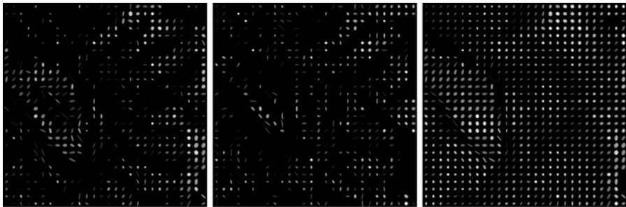
Fig. 22.4. (a) Left: white top hat with DSE(\sqrt{5}) . (b) Middle: black top hat with DSE(\sqrt{5}) . (c) Right: self-dual top hat with DSE(\sqrt{5})
