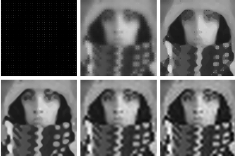
Fig. 19.2. Scalar-valued interpolation of Fig. 19.1(b). (a) Top Left : Interpolation data. (b) Top Middle : Interpolation with linear diffusion. (c) Top Right : Isotropic nonlinear diffusion. (d) Bottom Left : Anisotropic nonlinear diffusion. (e) Bottom middle : Biharmonic smoothing. (f) Bottom right : Triharmonic smoothing
