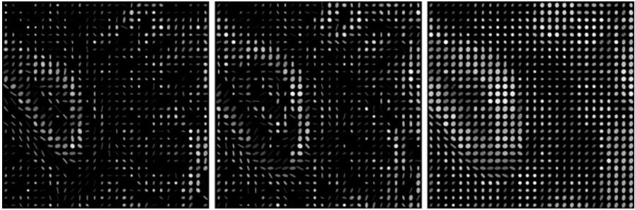
Fig. 22.5. (a) Left : external gradient with DSE(\sqrt{5}) . (b) Middle : internal gradient with DSE(\sqrt{5}) . (c) Right : Beucher gradient with DSE(\sqrt{5})
