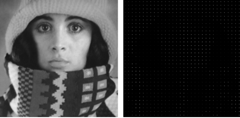
Fig. 19.1. (a) Left : Original image. (b) Right : Data points for interpolation. Only 1 out of 64 points is used
