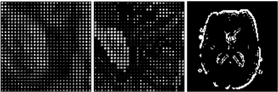
Fig. 22.6. (a) Left : morphological Laplacian with DSE(\sqrt{5}) . (b) Middle : result of shock filtering with DSE(\sqrt{5}) . (c) Right : edge map derived from zero crossings of the morphological Laplacian with DSE(\sqrt{5})
