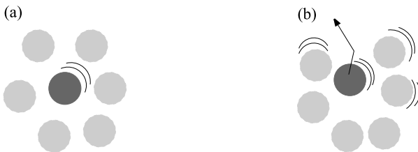
Fig. 16.4. Schematic view of a particle cage around a colloidal sphere for (a) short times \tau_B \ll t \ll \tau_I and (b) long times t \gg \tau_I .
