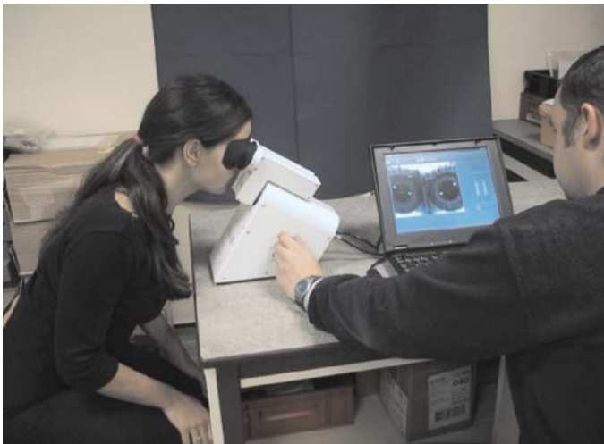
Fig. 11.9 Pupil diameter measurement using infrared technologies (P2000, Procyon): 10 pictures in a 2-s sequence
