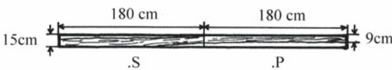
Fig. 10.33. Air-dried western hemlock, lumber section 9x9 cm. Relationship between stress and acoustic emission counts during a bending test until failure. P Zone of timber sample with straight grain; S zone of timber sample with slope of grain; 1.P acoustic emission counts on specimen 1, zone P ; 1.S acoustic emission counts on specimen 1, zone S , etc. (Nakagawa et al. 1989, with permission)
