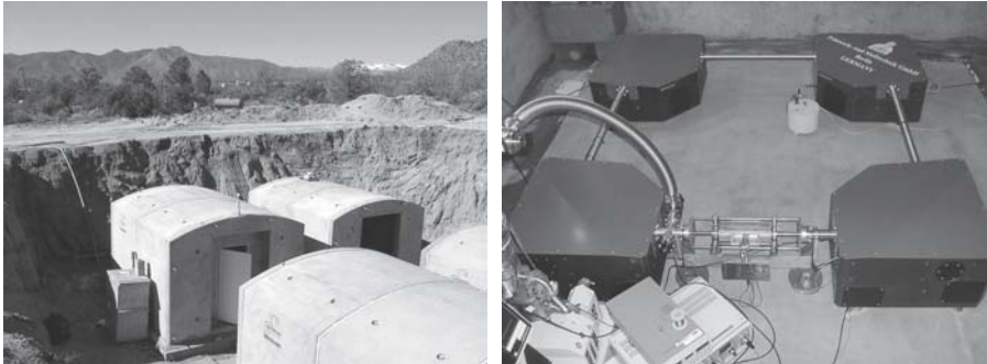
Fig. 4. The ring laser vault at the Pinon Flat (CA) observatory and the GEOSensor installation in one of the chambers
