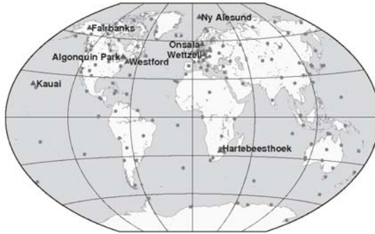
Fig. 1. Station networks: dots: GPS only; triangles: co-location VLBI and GPS
