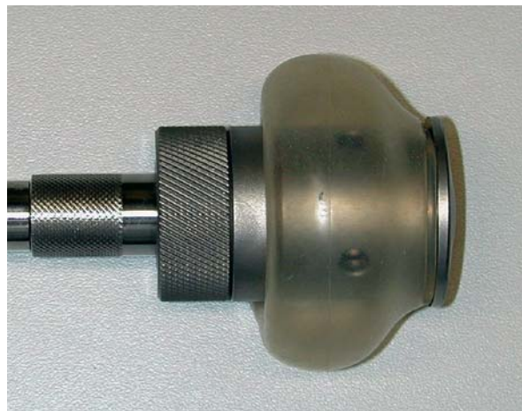
■ Fig. 6.12. Provisional pressuriser – sponge-filled sterile glove inserted by hand
