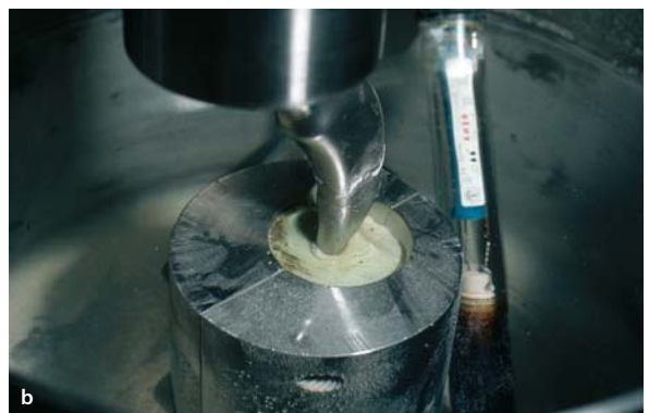
■ Fig. 3.55. a Highly-polished Exeter stem in a fatigue testing machine in Ringer's solution at body temperature. After 3 million cycles corrosion and microfractures of the sheath are visible. The bone cement had been vacuum mixed and pre-pressurised; 50 Hz, 3,5 kN. b Undulated stem surface in a vacuum-mixed and pre-pressurised cement mantle in Ringer's solution at body temperature revealing an intact interface after 55 million cycles; 50 Hz, 3,5 kN
