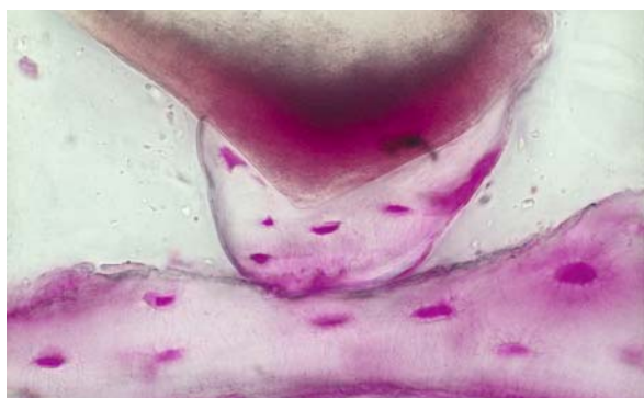
■ Fig. 3.60. Newly formed bone bonding directly on a ceramic particle adjacent to the bone-to-cement interface. Cross section through a rabbit's femur filled with bone cement containing Al_2O_3 ceramic particles. LM: fuchsin staining. 6 months after implantation
