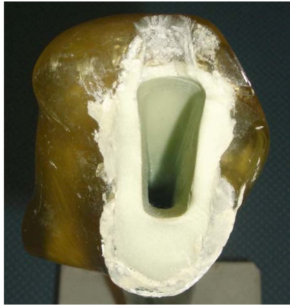
■ Fig. 7.22. Sawbone with a homogenous cement mantle after prosthesis explantation
