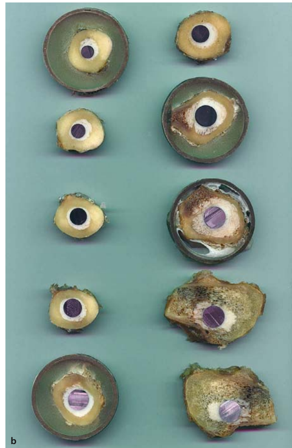
Fig. 8.29. a Transverse cuts of a cadaveric femur with »thin« cement showing the presence of windows at various locations. b As in a but with thick cement. (Note in both specimens on some slices the epoxy resin used to surround the femur to enable cutting is still in place)
