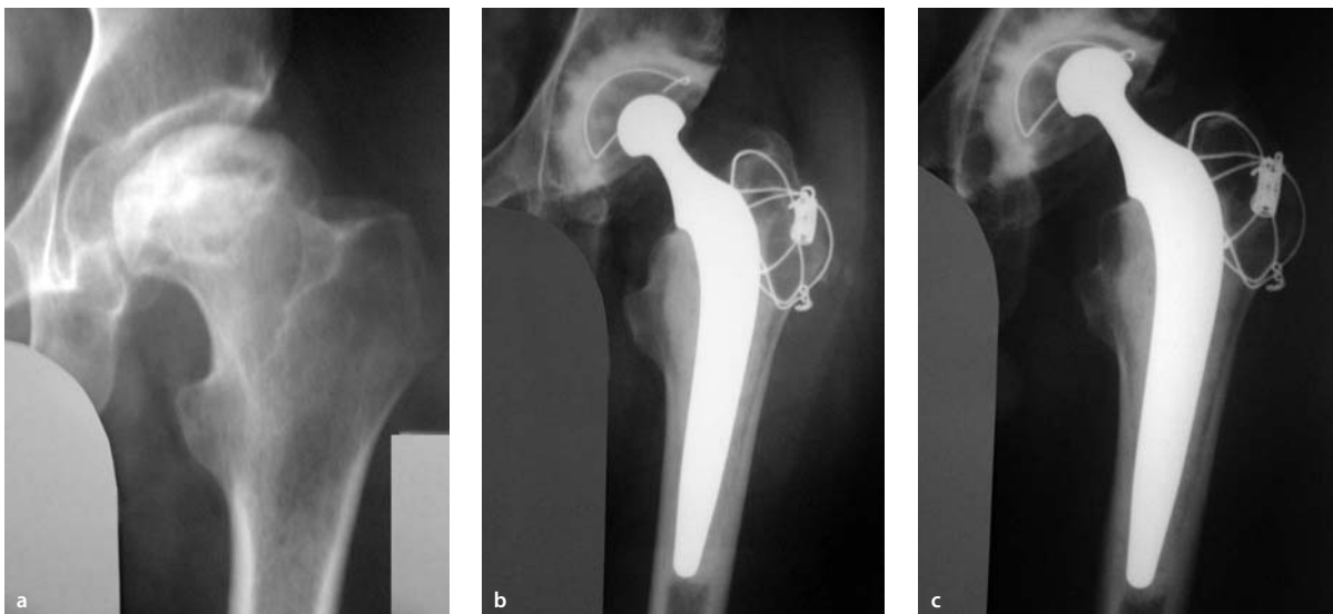
Fig. 8.6a–c. Penetration of the UHMWPE cup and no femoral cavitation. a Pre-operative radiograph, b Post-operative radiograph at 1 year, c radiograph at 18 years follow-up
