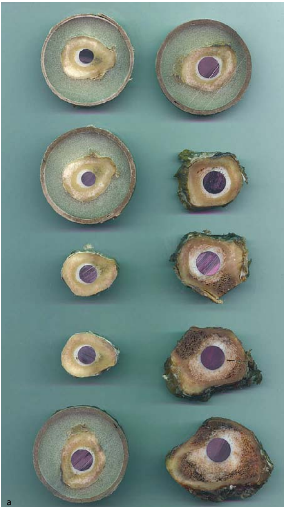
Fig. 8.29. a Transverse cuts of a cadaveric femur with »thin« cement showing the presence of windows at various locations. b As in a but with thick cement. (Note in both specimens on some slices the epoxy resin used to surround the femur to enable cutting is still in place)
