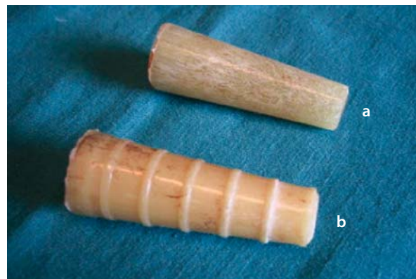
■ Fig. 3.20. Conical cement shells (a) before testing (b) after testing showing «bands» caused by outward creep of cement
