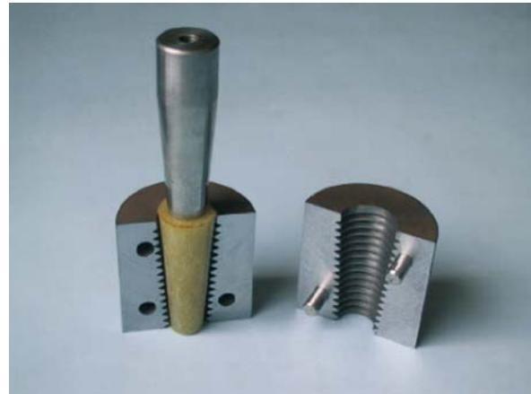
■ Fig. 3.19. Conical cement shell inside a grooved constraint before testing
