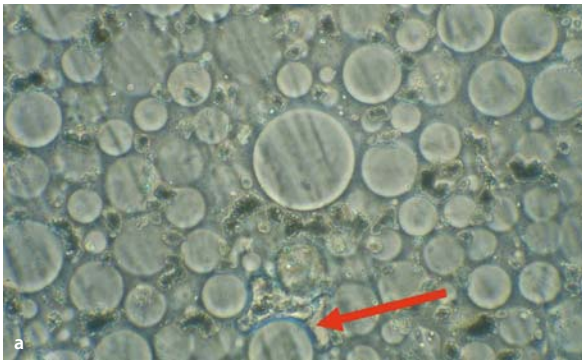
Fig. 3.46. a Cross section of a bone cement sample in the phase contrast: The mixture was exposed two minutes to a pressure acting on it of 3,5 Bar. The included air bubble, visible as a light blue line , is deformed ( arrow ). All beads reveal a dense ring around their circumfe-
