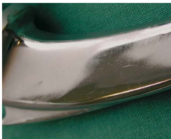
■ Fig. 7.1. Photograph of retrieved stem at revision for infection. Note burnishing and self-polishing at the (matt) stem surface
