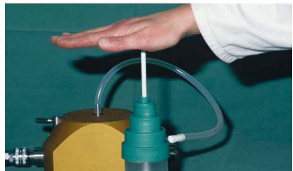
Fig. 3.48. Vacuum-mixing system investigated with ideal-diameter mixing bowl. The Teflon-coated rod does not adhere to PMMA bone cement thus avoiding inhomogeneity of the mixture and air inclusions leading to macroporosity during mixing
