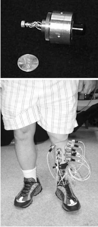
Fig. 9.3. Example of interface stress measurement system. With this system pressures and shear stresses are monitored at 13 socket sites during standing or walking. The transducers and mounts are small and lightweight (<25 g) so as to minimize weight addition to the prosthesis
