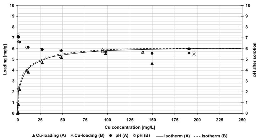
**Fig. 1.** Isotherms of the loading of the Biocer material with Cu<sup>2+</sup> in tap water (unbuffered, initial pH 4.5).
