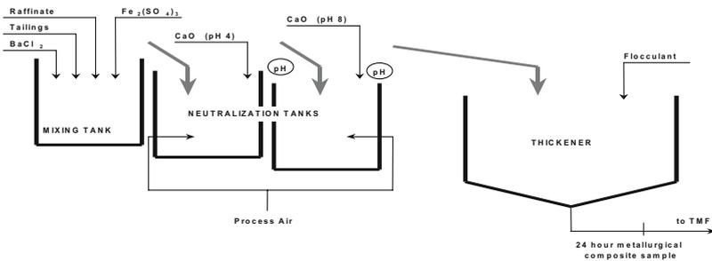
Fig. 1. Diagram of Tailings Neutralization Circuit – JEB Mill.
