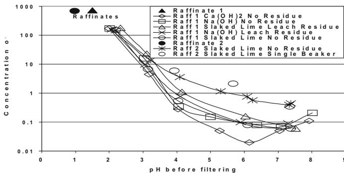
Fig. 2. Arsenic concentrations during raffinate neutralization experiments.
