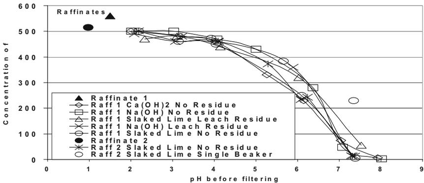
Fig. 3. Nickel concentrations during raffinate neutralization experiments.
