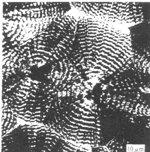
Fig. 7.14 Spherulites of polyethylene. 20) [Reproduced with permission from N. Kasai, K. Kobayashi, Structure and Properties of High Polymers , p.110, Maruzen (1963)]
