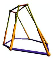
From the measurements of the length of the arms, we would like to know the position of the platform. This problem is a classical benchmark in polynomial system solving. We know from [RV95, Laz93, Mou93] that this problem has at most 40 solutions and that this bound is reached [Die98]. Here is the 40 degree curve that we obtain when we remove an arm of the mechanism:
