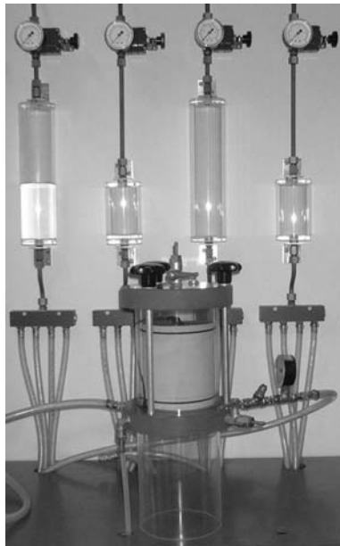
Fig. 5.19. Experimental set-up of the DARCY experiment, applied to samples of the field-block rock matrix.
