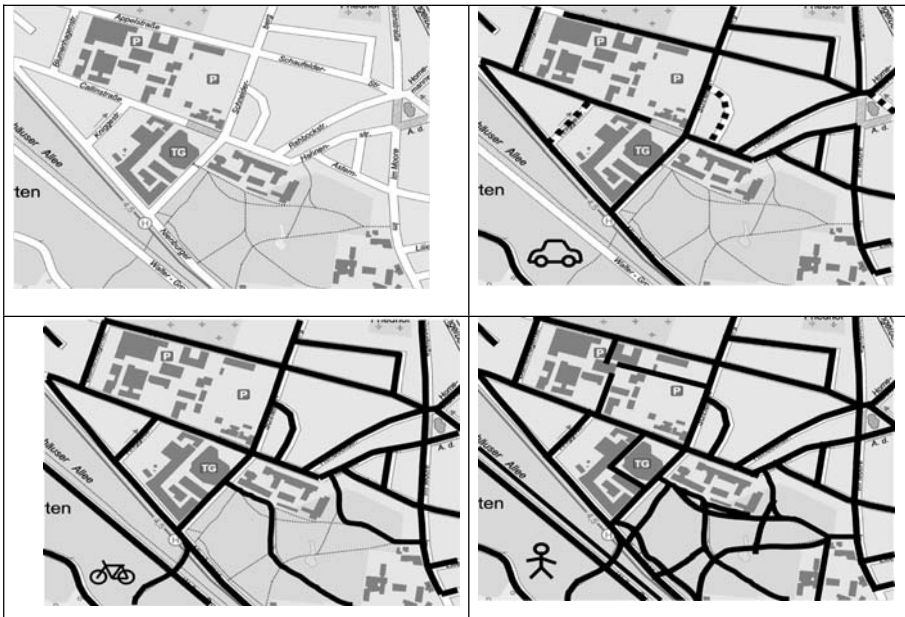
Fig. 6.1. City plan (upper left); Graphs for route processing depending on moving mode: by car (upper right), by bicycle (lower left), on foot (lower right)
