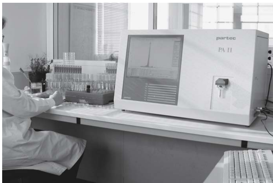
Fig. 1. Ploidy level determination of anther culture-derived plantlets by flow cytometry. Thirty plants can be checked in 1 h to identify spontaneous doubled haploid plantlets and to ensure an efficient chromosome doubling of haploid plants at an early stage
