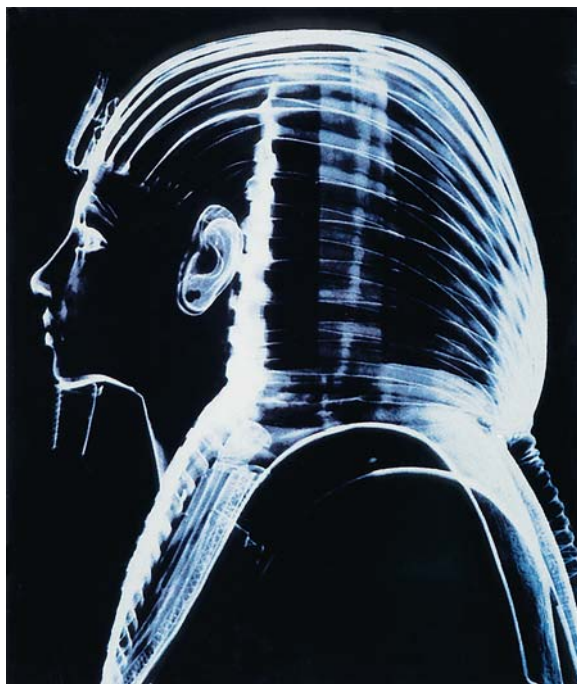
Fig. 8.9. Gamma radiography of the gold mask of Tutankhamon made for the Exhibition “Toutankhamon et son Temps”, Paris 1967. © Rights reserved
