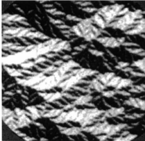
Fig. 6.15. SPLEEM image of the magnetic domain structure of a Co(0001) surface taken with 2 eV electrons. Field of view 12 \mu\text{m}
