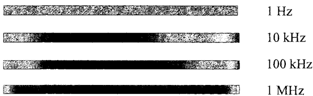
Fig. 14.7. Current density in the outer left conductor for four different frequencies. As frequency increases the current concentrates at the edges of the conductor. The dark color in the middle of the conductor represents low current density
