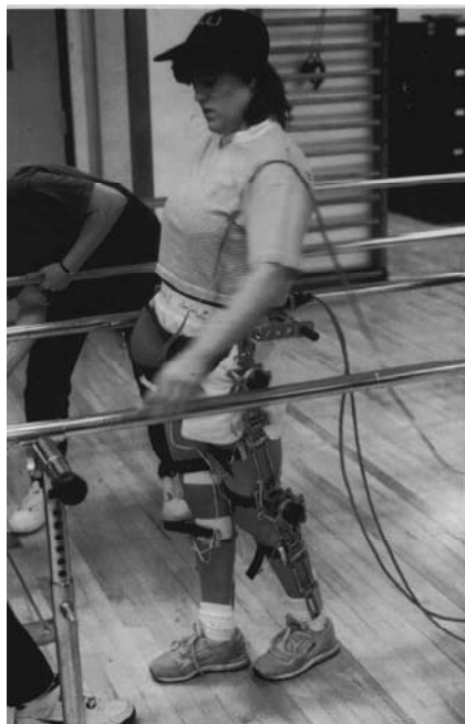
Fig. 2. User is paralyzed from the waist down following a T10 complete spinal cord injury. Rudimentary gait, using parallel bars for balance, is realized by electrical stimulation of the paralyzed muscles. This hybrid system combines the stimulation with a mechanical orthosis.
