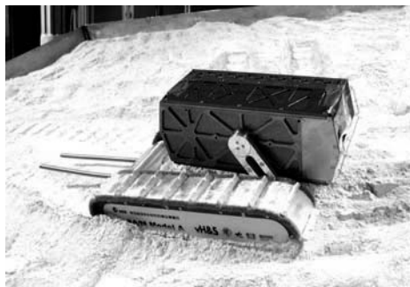
Fig. 3. The Nanokhod micro-rover for planetary exploration, developed by the European Space Agency
