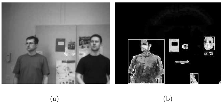
Fig. 4. Original image (left) and Skin-filtered image (right). Detected outlines are marked, valid face candidates are indicated by boxes.
