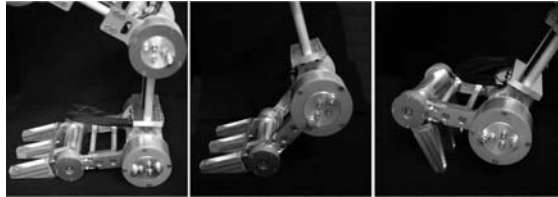
Fig. 3. Current Leg Configuration inspired by Four Legged Mammals.
