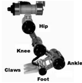
Fig. 3. Current Leg Configuration inspired by Four Legged Mammals.
