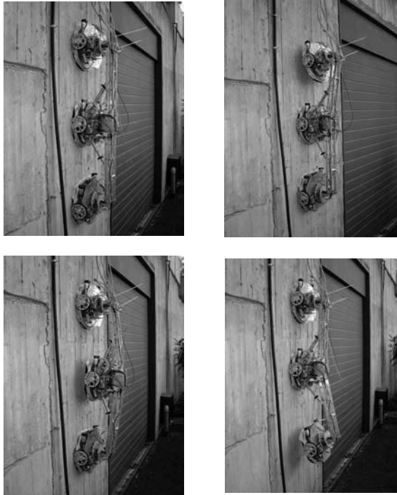
Fig. 4. Steps sequence for passing over an obstacle
