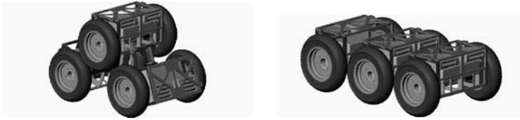
Fig. 1. MiniRoc in a 4 wheels (left) and 6 wheels (right) configurations
