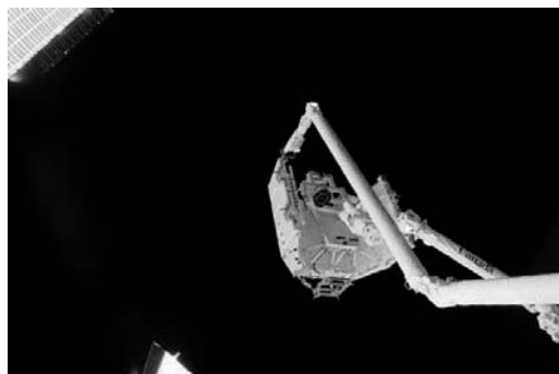
Fig. 2. Hand-over of large object from Space Shuttle to Space Station robot.
