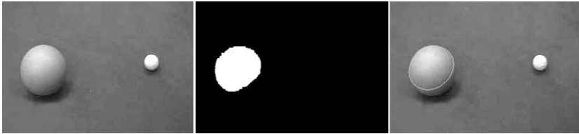
Fig. 2. The original image, image thresholded with orange color and the found orange circle [9]
