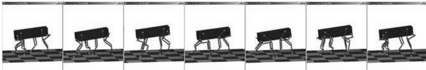
Fig.5 Trot locomotion of movement simulator.
