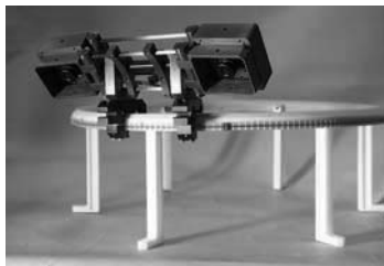
Fig. 4. Camera track assembly allows the stereo cameras to rotate through 360^\circ
