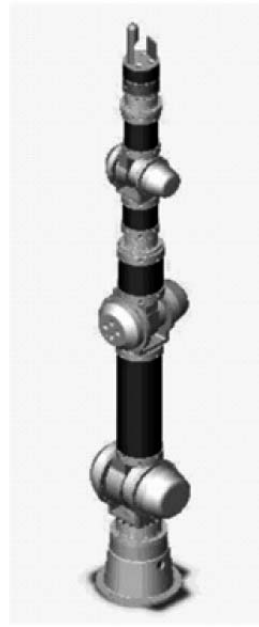
Fig. 3. Manipulator LWR-UC3M1 modelled with SolidWorks®.
