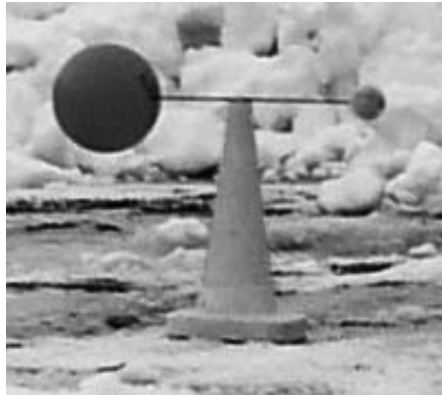
Fig. 1. A passive sign placed in one corner of the working area. The sign is pointing in to the direction of the next corner point. The position vector pointing from the center of the big ball to the center of the small ball defines the direction.
