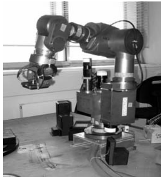
Fig. 1. 7-axis revolute joint ANSALDO arm
