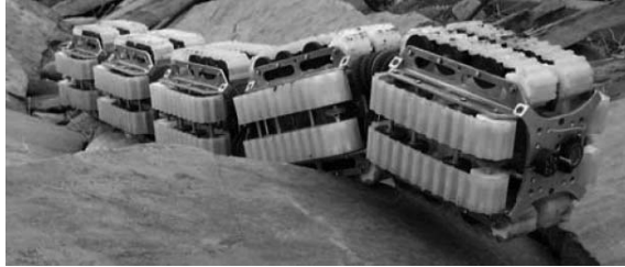
Fig. 2. The OmniTread serpentine robot. All segments are linked by 2-DOF pneumatically actuated joints, which are the focus of this paper.
