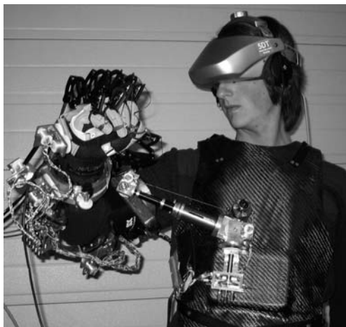
Figure 5: Telepresence MMI for EUROBOT (includes single arm exoskeleton)
