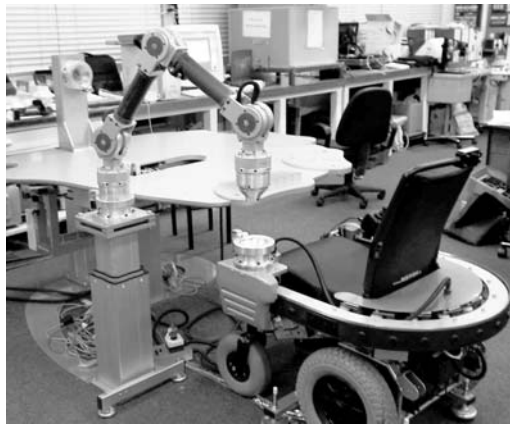
Fig. 2. The robot is able to transfer from the environment to the wheelchair.
