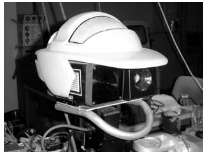
Fig. 3. Robot head includes camera, laser pointer and five LEDs.
