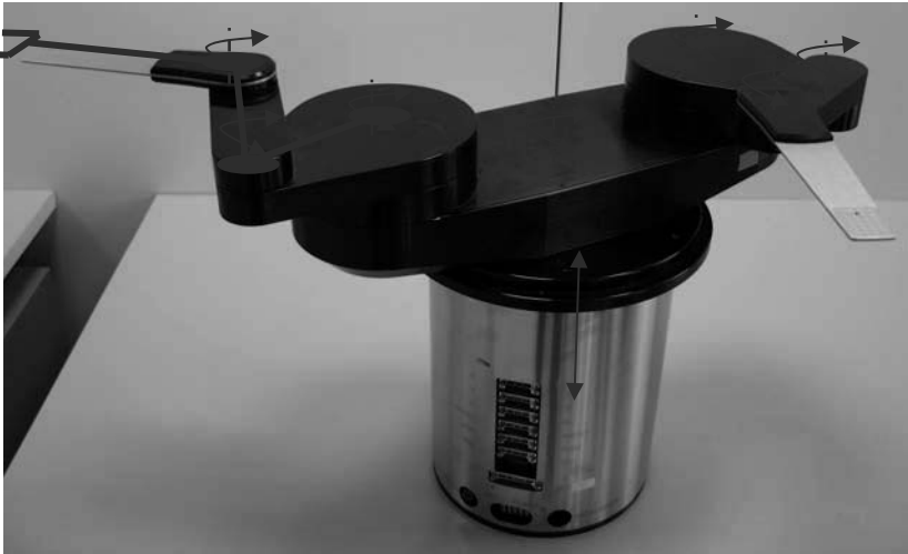
Fig. 4. The manipulator adopted in the Cleaning Room for 6" Wafer Manipulation.
