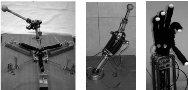
Fig. 9. The view of two arms manipulator with 4 DOF and an artificial hand
