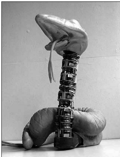
Fig. 5. Serpent with actuated “neck” before colouring.
