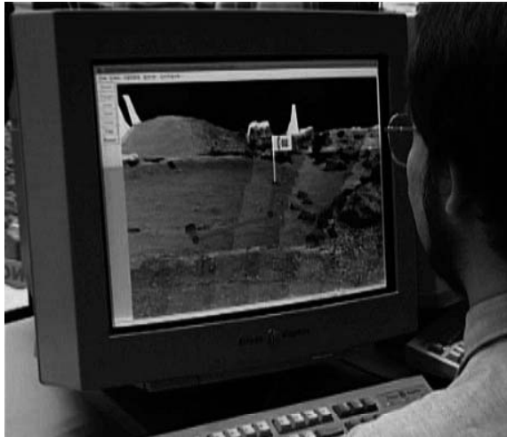
Fig. 6. Example of operator control through a high-level abstraction user interface.
