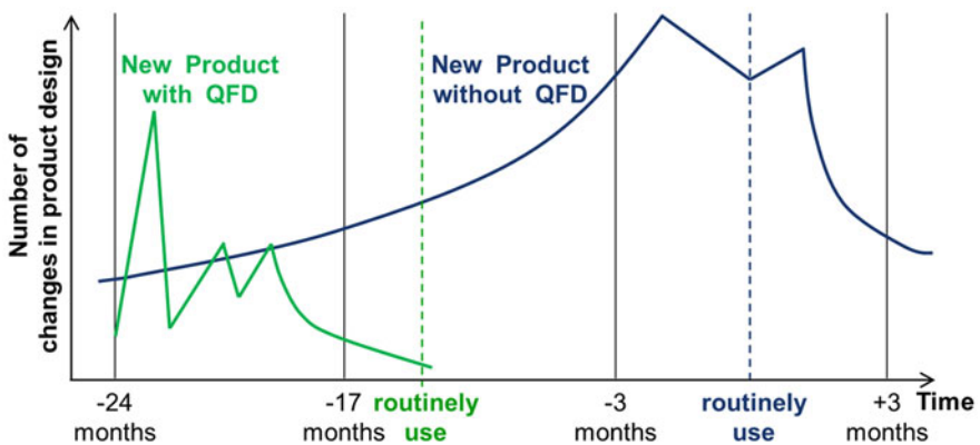
Fig. 1 Impact of quality function deployment in industry. The higher efforts and costs of structured product planning with quality function deployment (QFD) in the beginning of a car development are counterbalanced by shorter development times and less flaws of the product following start of production. Transfer to in vitro model and test method development should reduce the time-to-application similarly, from Zoschke (1993)
