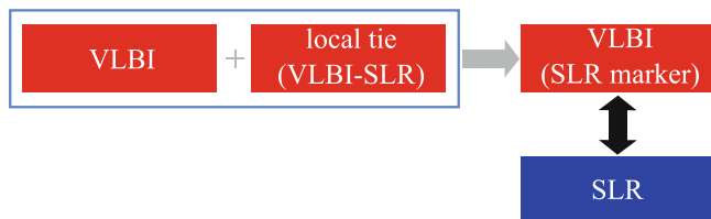
Fig. 2 Direct comparison of DGFI-TUM’s VLBI and SLR single-technique solutions by using local ties between co-located instruments
