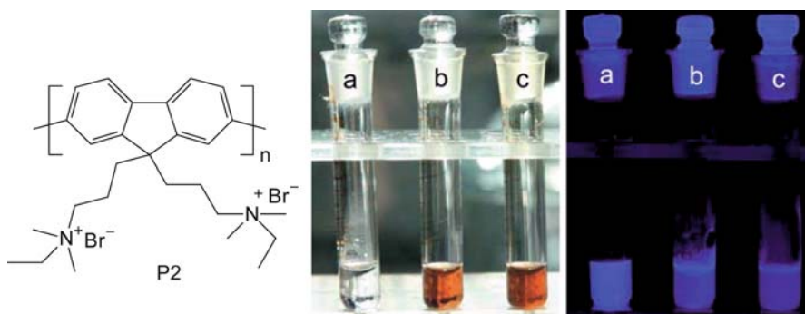
Fig. 8 Left : A chemical structure of poly(9,9-bis{3'-(( N,N -dimethyl)- N -ethylammonium})-propyl}-2,7-fluorene dibromide) (P2). Right : A photograph of P2 with different concentrations in water ( left ). A photograph showing emission of light from P2 with different concentrations in water, the photograph was taken under irradiation with light at 365 nm ( right ). (a) Dilute solution ( 1 \times 10^{-3} mg/mL), (b) 50 mg/mL, (c) 100 mg/mL. Reprinted with permission from [42]. © (2007) by Wiley-VCH Verlag GmbH & Co. KGaA
