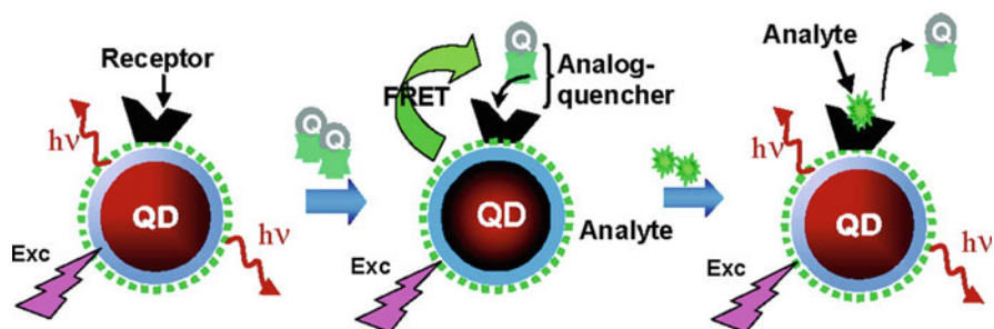
Fig. 6 Schematic illustration of a QD-based FRET competition assay for TNT detection. (Reprinted with permission from [42]. Copyright 2005 American Chemical Society)
