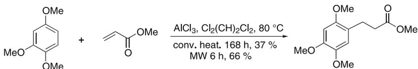
**Scheme 7** Microwave-assisted synthesis of methyl 3-(2,4,5-trimethoxyphenyl)propionate
