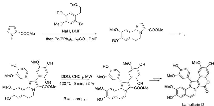
**Scheme 23** Total synthesis of Lamellarin D
