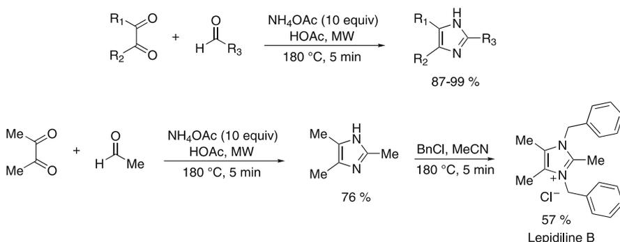
**Scheme 18** Microwave-assisted synthesis of Lepidiline B
