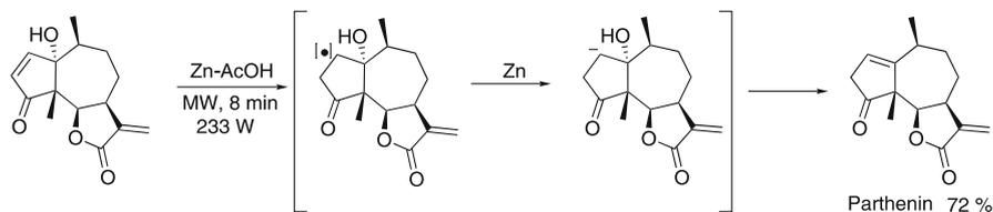
**Scheme 27** Microwave-assisted modification of Parthenin
