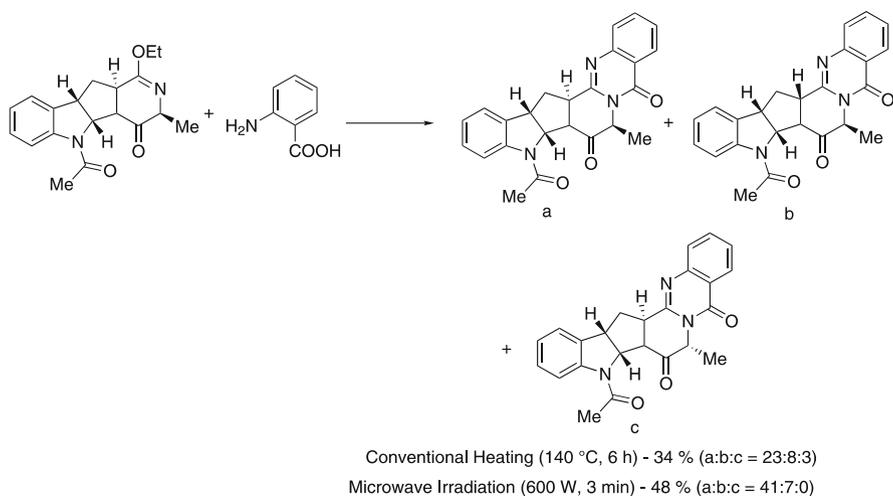
**Scheme 42** Microwave-assisted synthesis of de-Prenylardeemins
