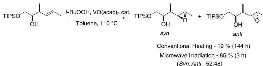
**Scheme 44** VO(acac)<sub>2</sub>-catalyzed epoxidation; conventional heating versus microwave irradiation
