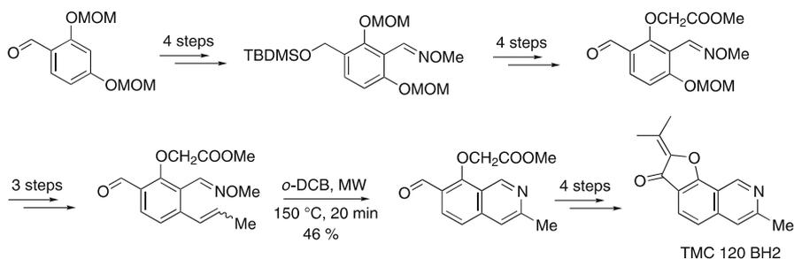
**Scheme 14** Microwave-assisted synthesis of alkaloid TMC 120B
