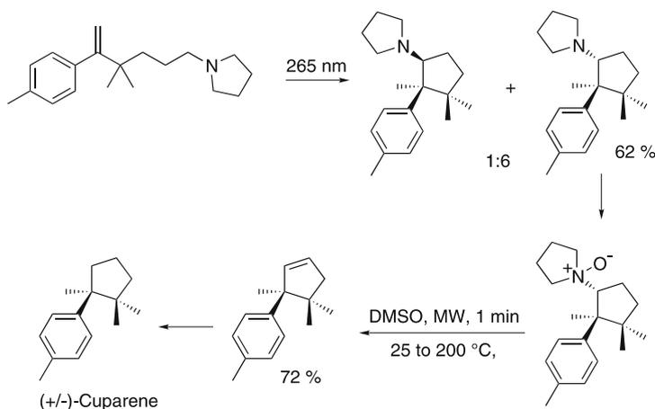
**Scheme 9** Photomediated and microwave-assisted synthesis of Cuparene
