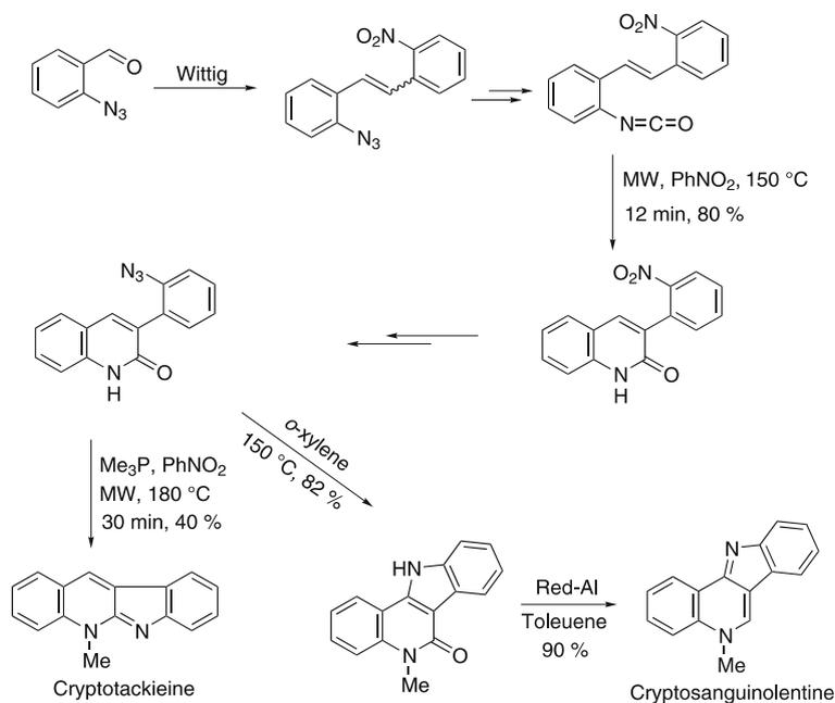
**Scheme 13** Microwave-assisted synthesis of Cryptotackieine and Cryptosanguinolentine
