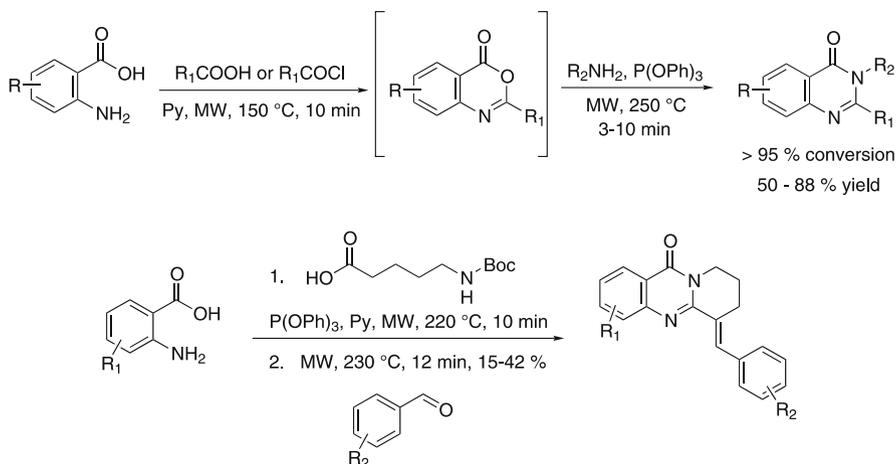
**Scheme 19** Microwave-assisted one-pot synthesis of 2,3-disubstituted 3*H*-quinazolin-4-ones
