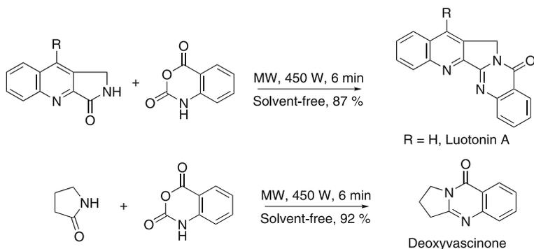
**Scheme 16** Microwave-assisted synthesis of Luotonin A and Deoxyvascinone
