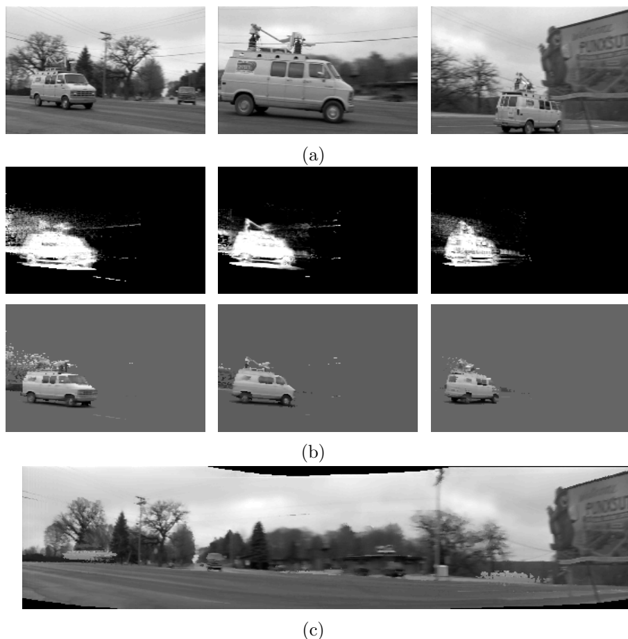
Fig. 4. Panel (a) shows three frames of the van sequence. Panel (b) shows the pairs of mask and the element-wise product of the mask and appearance (showing against a grey background) for all different viewpoints. Note that the element-wise products are produced by making the masks binary (thresholded to 0.5). Panel (c) displays the background.
