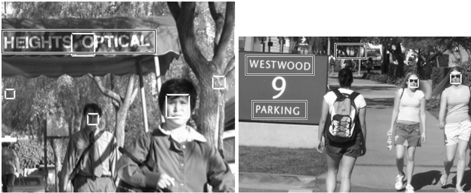
Fig. 11. The boxes show faces and text as detected by the AdaBoost log posterior ratio test with fixed threshold. Observe the false positives due to vegetation, tree structure, and random image patterns. It is impossible to select a threshold which has no false positives and false negatives for this image. As it is shown in our experiments later, the generative models will remove the false positives and also recover the missing text.
