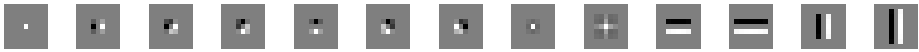
Fig. 2. The bank of 13 filters. From left to right, they are: a delta function, 6 oriented Gaussian derivatives, a Laplace of Gaussian, a corner detector, and 4 bar detectors.
