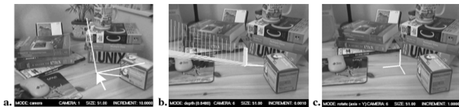
Fig. 5. Insertion of the virtual frame into a desk scene: a) initial placement into one of the reference images by specifying the desired location of the frame’s origin; b) the frame’s trajectory along the epipolar line in another image; c) subsequent orientation adjustment
