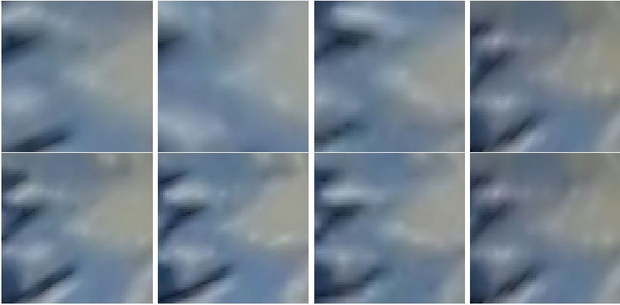
Fig. 6. Refining patch parameters across multiple views: rectified patches associated with a match in four views before (top) and after (bottom) applying the refinement process. The patch in the rightmost column is used as a reference for the other three patches. The errors shown in the top row are exaggerated for the sake of illustration.
