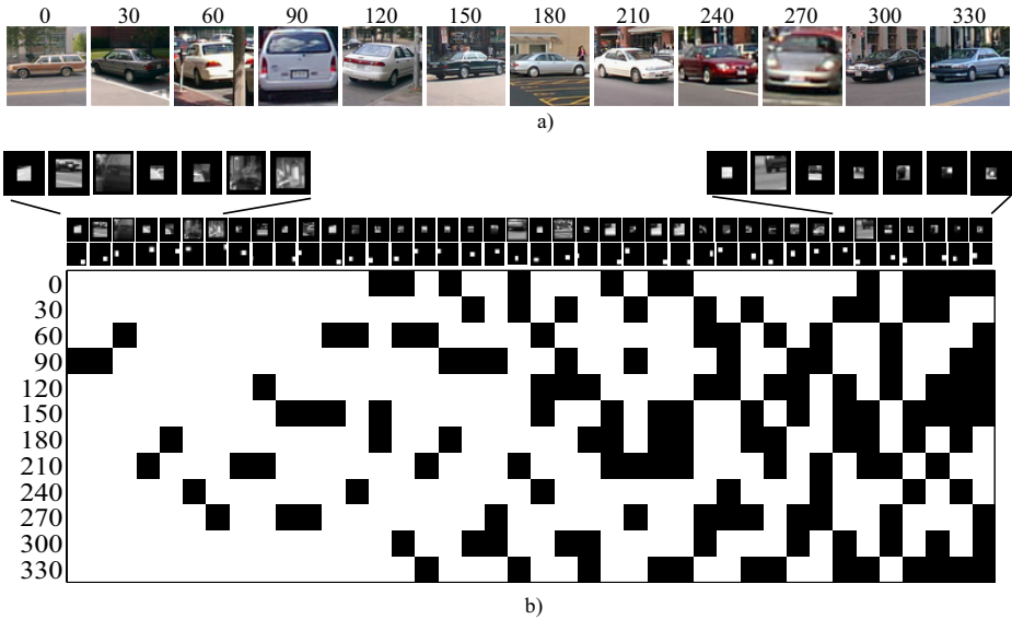
Fig. 10. Matrix that relates features to classifiers, which shows which features are shared among the different car views (orientation is discretized in 12 groups). The features are sorted from left to right from more generic (shared across many objects) to more specific.
