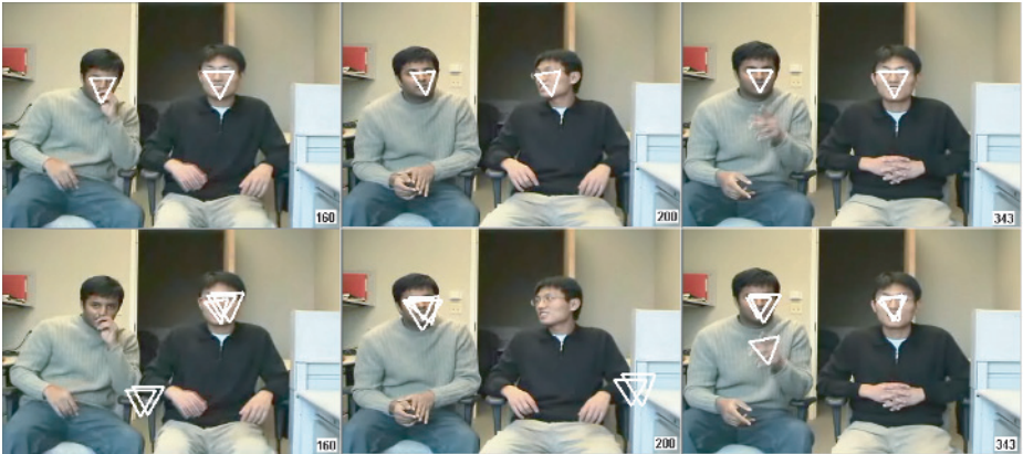
Fig. 8. Top row: The result of our tracker in three different frames. Bottom row: The raw results of pure detection in the same three frames.
