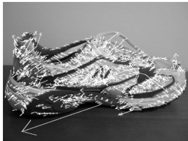
Fig. 2. SIFT keypoints extracted from a 640 \times 480 image of a sneaker. The algorithm found 1533 features shown as white arrows, with size and direction corresponding to feature scale and orientation, respectively.
