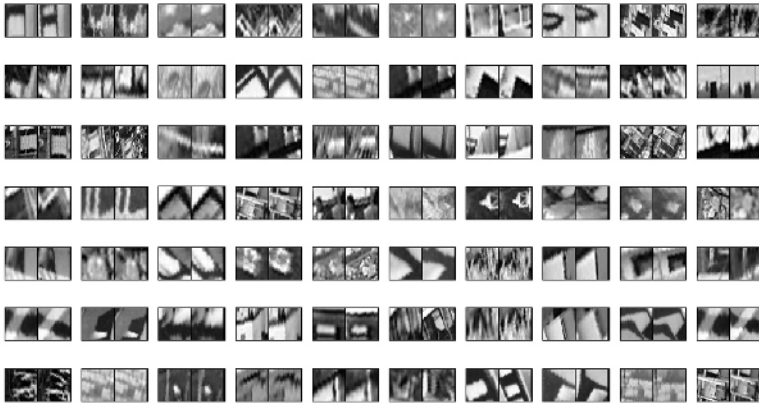
Fig. 5. Rectified paired patches found by the Harris-Affine detector. Note that the centers of the patches are usually on edges or at corners, and that the orientations and scales of matched patches are often slightly different.
