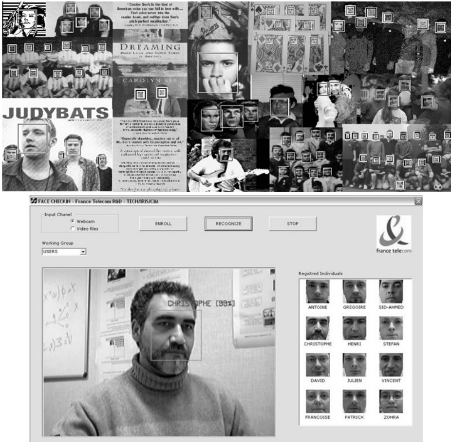
Fig. 1. Some results of CFF on the CMU test set and a CFF-based face recognition system at France Telecom
