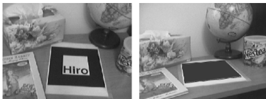
Fig. 10. ARToolkit marker in the scene (left). Virtual square, superimposed onto the marker during tracking (right).
