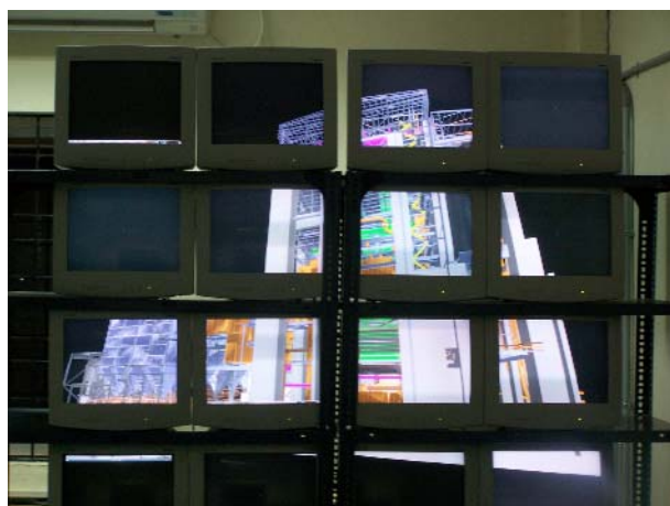
Fig. 7. A 4×4 display wall rendering of UNC’s Powerplant. The combined resolution is 12 MPixels. Efficient rendering to a display wall requires fast visibility culling of the scene to all the frustums. Adaptive culling by merging of the object and frustum hierarchies makes this possible for even bigger tile configurations.
