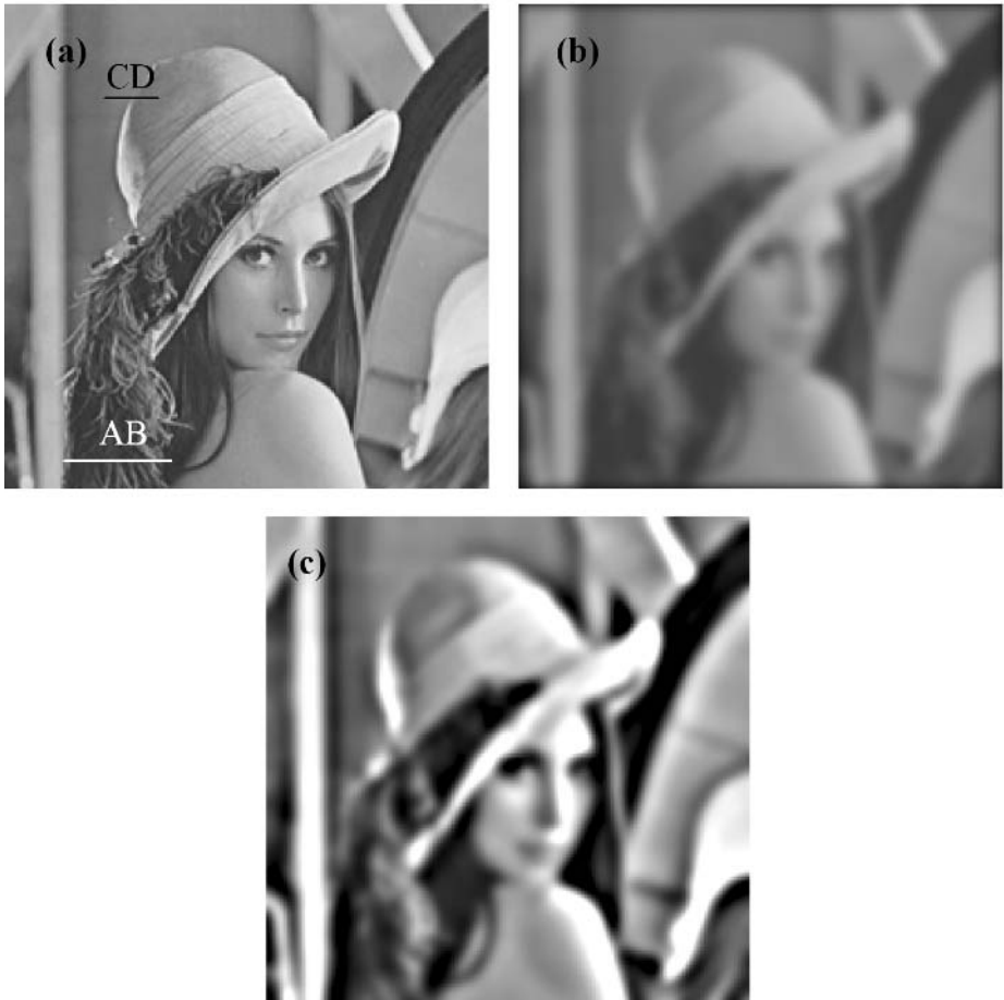
Fig. 12. (a) The benchmark image of Lena. (b) The resultant image when (a) is convoluted with a Gaussian function. (c) The resultant image when (a) is convoluted with the MDoG function.
