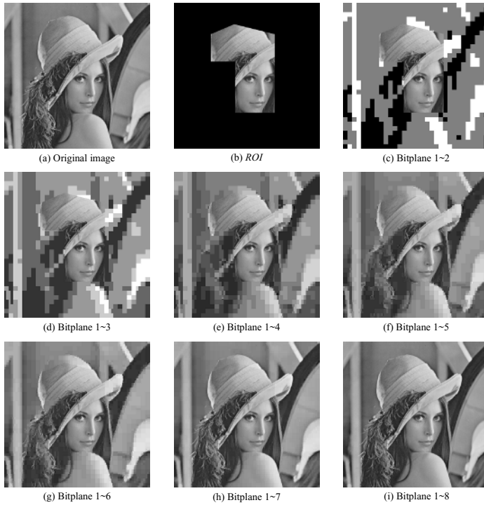
Fig. 5. Progressive lossy-to-lossless coding with polygon-shaped ROI
