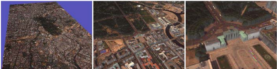
Fig. 8. Automatically generated 3D model of Berlin (different zoomings)
