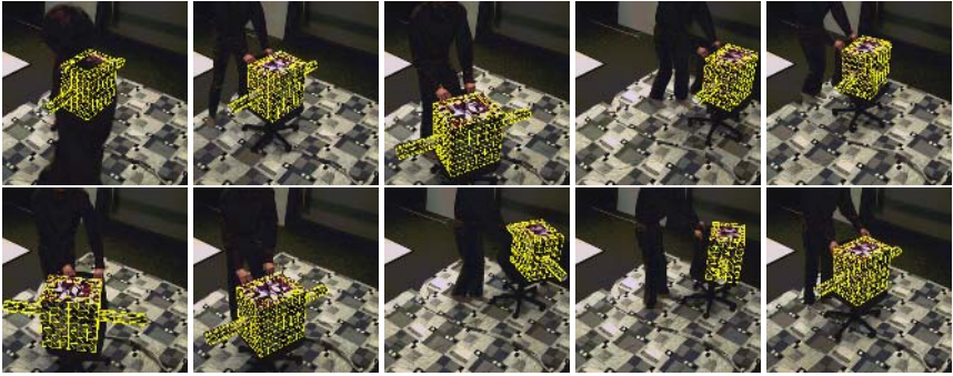
Fig. 8. Pose estimates for 10 of 570 frames. The sequence contains several difficulties for tracking: a rich textured and non-static background, shadows, occlusions, and other moving objects. Only one camera view is shown.
