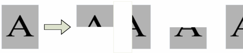
Fig. 2. Block matching method. The four blocks represents the fact that an occlusion always happens from one side of the target, left, right, up or down.
