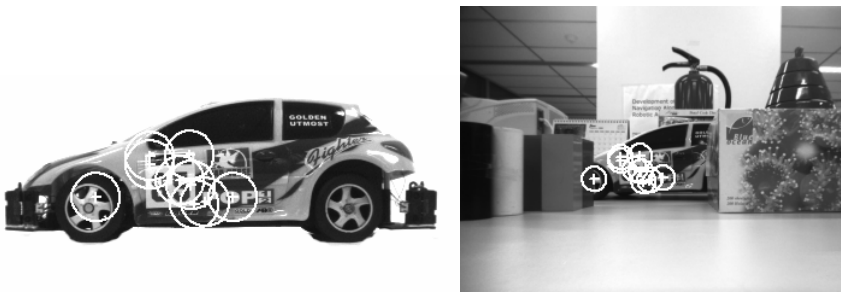
Fig. 1. Correctly selected scales for matching local features in both images (from [5])
