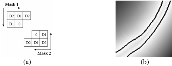
Fig. 5. Distance map (a) forward and backward masks (b) the result of chamfer distance map
