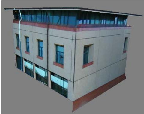
Fig. 7. Triangulated surface mesh with textures
