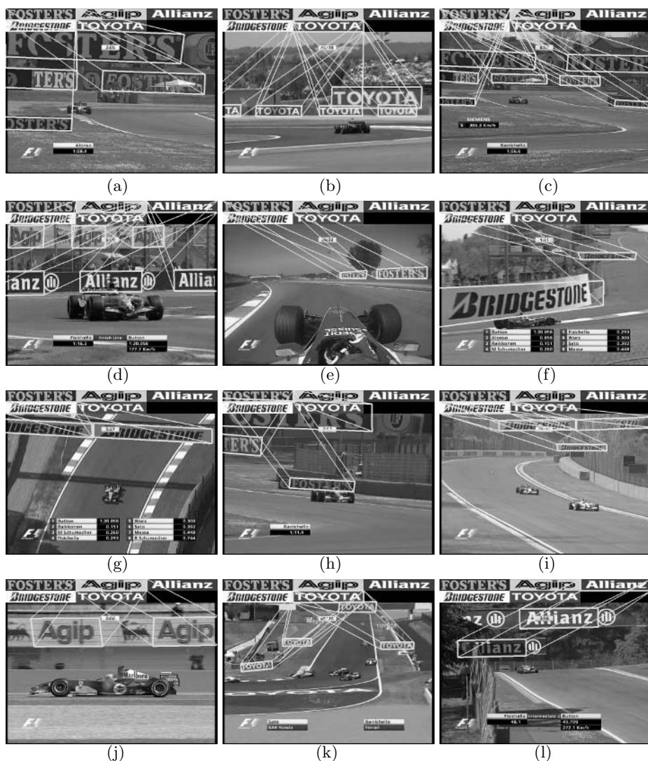
Fig. 4. Recognition results for broadcasts of F1. The rectangles in the figures show the recognition results. Figures (a) to (j) show successful cases. In spite of deformations, illumination changes and occlusions of the ads in these scene images, all ads were successfully recognized by separating point correspondences of each instance. These results demonstrate that our method recognizes multiple ads in various situations even if only one model image is given. Figures (k) and (l) show failure cases. (k) Since the ranges of deformation and scaling that could be covered by the invariants were exceeded, point correspondences could not be obtained for the ad on the ground in front and the small ads in distance. (l) The degree of occlusion was large and recognition of the top left ad failed. Such failures may be eliminated by improving the local invariant features and using several model images including the deformations of targets that can be expected beforehand.
