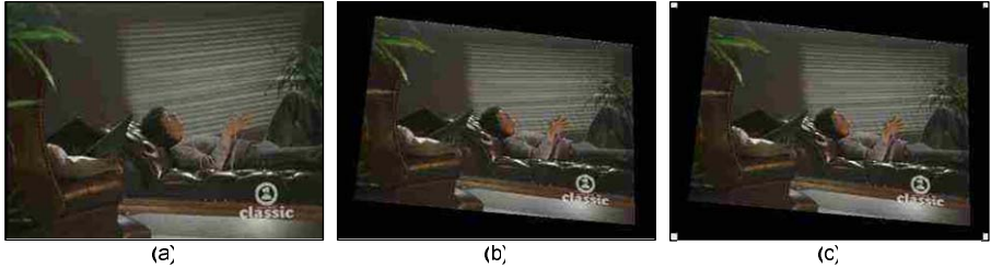
Fig. 9. Warping processing: (a) input image, (b) pre-warp image, and (c) add corner points to a pre-warp image
