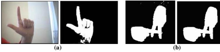
Fig. 2. (a) Original image and detected skin regions after pixel classification, (b) result of the morphological opening
