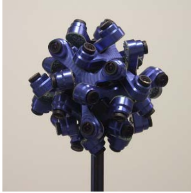
Fig. 2. Stereo Omni-directional System (SOS). 17cm diameter sphere consist of 36 CCD cameras.
