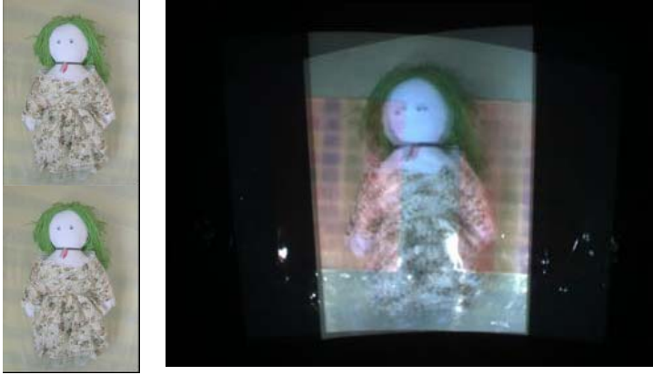
Fig. 6. Geometric and radiometric distortion. Left images: projector input images of two projectors, right image: projection by two projectors without any processing.
