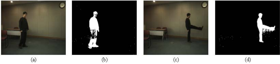
Fig. 1. Problems of the background subtraction method to extract human silhouettes. In (a) and (b) some parts of the human silhouette disappear when the color of these parts is too similar to that of the occluded background area. (c) and (d) shows the shadow problem. These silhouettes were obtained with the Horprasert's algorithm [6].
