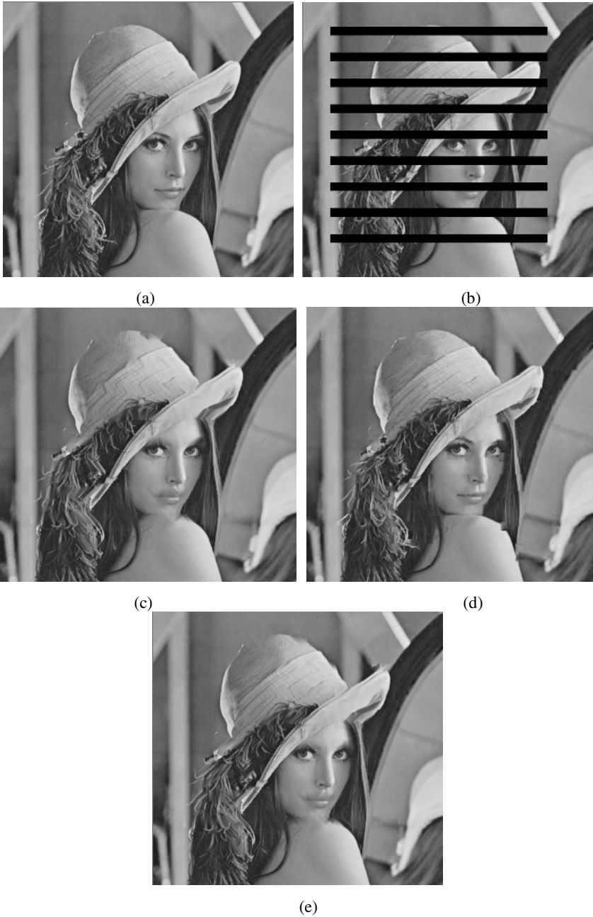
Fig. 9. Test results for Lena: (a) Original image (b) Damaged image (c) Hsia's (d) RIBMAP and (e) Proposed algorithm
