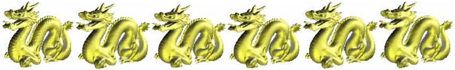
Fig. 10. The reconstructed results of the Dragon model on various levels after adopting the Depth First reduction. From left to right, Base model (90374points), reconstructed model (56302 points), 55287 points, 49663 points, 30832 points, and 13237 points (3% of original).
