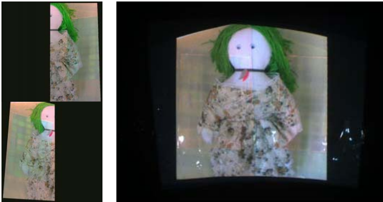
Fig. 8. An example of applying the proposed radiometric compensation method (using multiple overlapping projectors) to a non-Lambertian curved surface. Left images: projector input images which are partially compensated for compensating the whole image, right image: compensated projection image. The color of the whole projection image was successfully compensated except for artifacts due to the unevenness of the projection surface.
