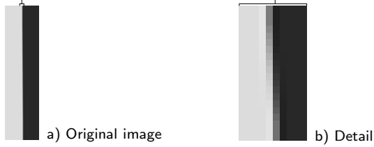
Fig. 4. Synthetic image used in the experiment. The edge is slightly slanted, so that feature points with a range of subpel coordinates can be detected.
