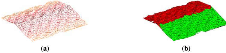
Fig. 3. Illustration of detection for roof planes (a) triangles mesh (b) extracted planes
