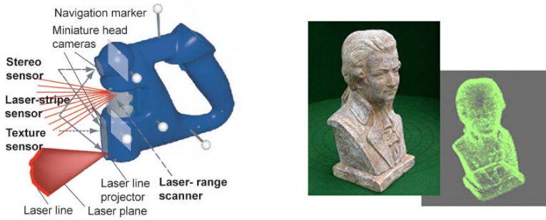
Fig. 1. DLR Multisensory 3D-Modeler and a scanned bust
