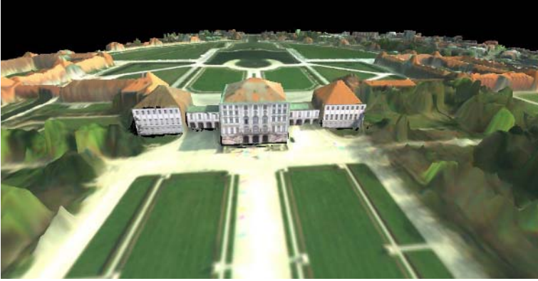
Fig. 9. Extracted 3D model of the DEM data (HRSC) with (partially) mapped textures captured by a terrestrial panoramic camera
