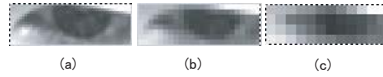
Fig. 5. Example images of an eye with (a) 16 \times 48 , (b) 8 \times 24 , and (c) 4 \times 12 pixels
