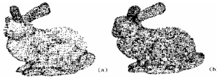
Fig. 2. The Bunny model (34838 points) as an example using different thresholds. When the coefficient f = 0.005 (a), the number of relevant points is 5616; when f = 0.001 , the number of relevant points is 12307 (b).
