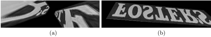
Fig. 3. Examples of appearances of ads that are rejected in RANSAC. (a) an appearance corresponding to a twisted rectangle, (b) an appearance corresponding to a reversed rectangle. Such appearances are never observed in actual scenes.
