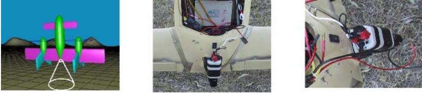
Fig. 1. Simulation drawing and photos of the camera set-up on the T-Wing
