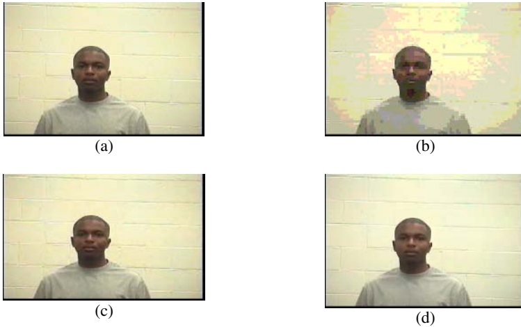
Fig. 6. Illustration of visual perception with 0.7% compression ratio. (a) original 9.5 meters face image; (b) JPEG; (c) JPEG 2000; (d) Vidware Vision TM .
