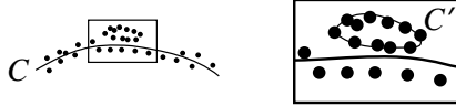
Fig. 2. A point sample satisfying sampling conditions (i) and (ii) for a single component curve C (left) and also the curve C \cup C' (right)
