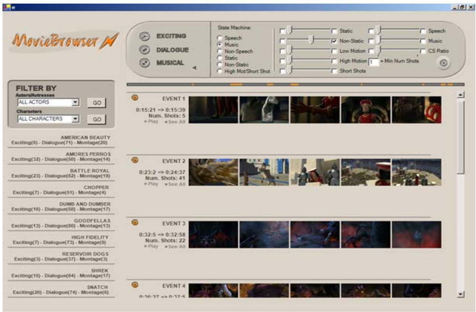
Fig. 3. Search-based browsing displaying the retrieved events after searching for events that contain high amounts of music and moving camera shots
