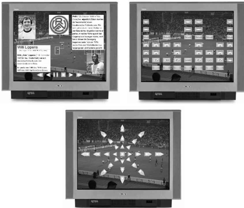
Fig. 3. Problem of interaction design: placing additional information (left), information about content structure (middle), interaction with the content structure (right)
