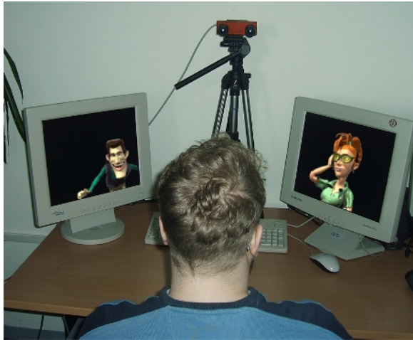
Fig. 7. The constellation of the second application showing two displays with different characters and the head tracker. Depending on which display the user is focusing the story continues differently.
