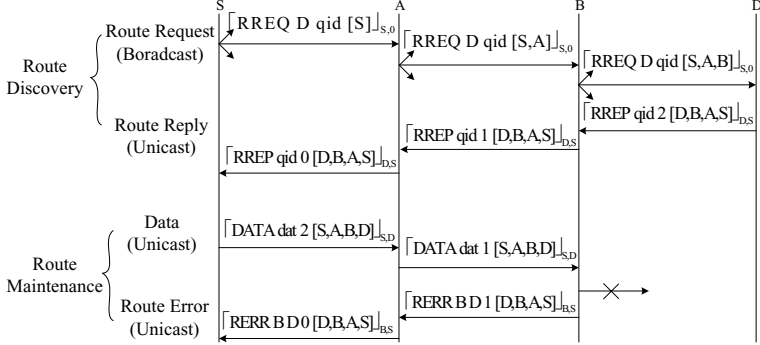
Fig. 2. The basic operation of DSR
