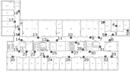
Fig. 9. Large scale experiment consisting of 40 nodes spread out on an office floor. Node 1 is the initiator of all data communication.
