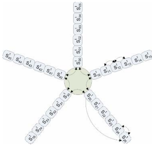
Fig. 5. The two-dimensional CA lattice. The arrows represent the interaction between a cell (possibly located somewhere in the middle or on the edge of the lattice) and its neighboring cells. Essentially the interaction is similar to the model in § 2 except modules closest to central disc interact with modules in similar position located on the neighboring leg.
