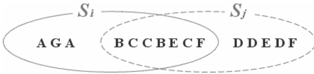
Fig. 6. The union bag of the two sequences S_i and S_j . The union value is the number of all elements.
