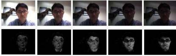
Fig. 6. Skin Color Area. The probability densities of the trained skin color model are calculated at all pixels and scaled for displaying.
