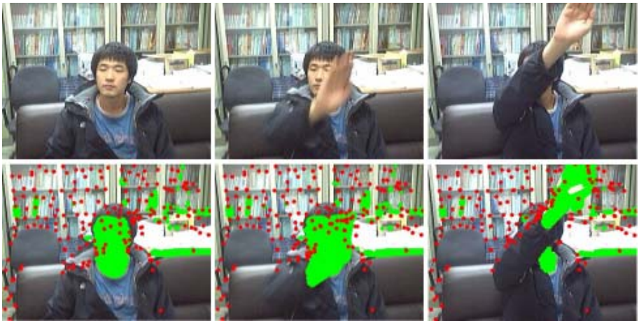
Fig. 2. Identifying hand gestures by filtering skin color regions and tracking feature points
