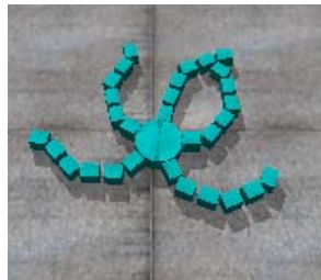
Fig. 7. Snapshot of the simulation for the robot using single transition rule for all the modules represented by a two-dimensional CA lattice
