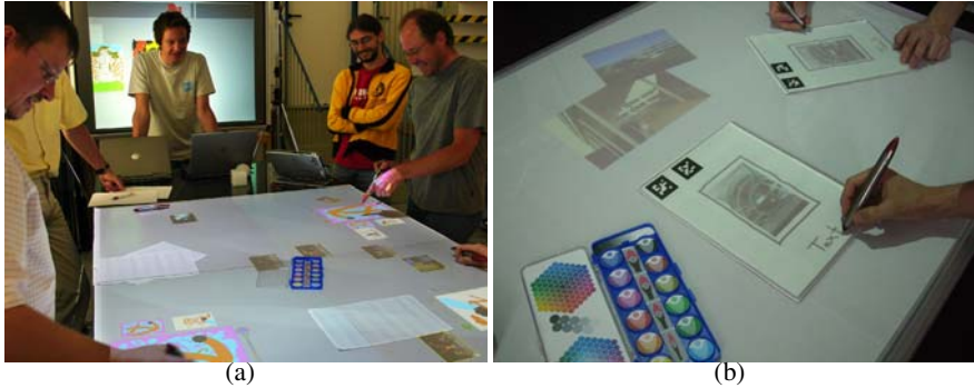
Fig. 1. (a) Participants can either interact with the interactive table either using tablet PCs or digital pens. (b) The collaboration mode allows to sketch the same document.
