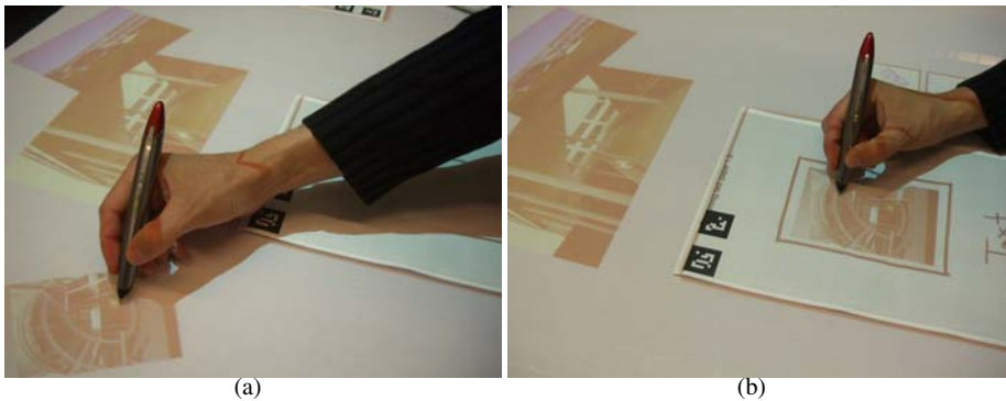
Fig. 7. Pick-and-Drop. Users can pick (a) an object from the interactive table to drop it (b) onto the real paper.
