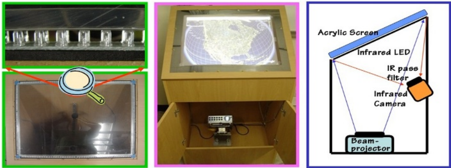
Fig. 3. The acrylic screen attaching infrared LED (left). The inside of the prototype system, and the configuration of camera and projector (right).
