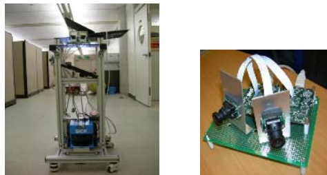
Fig. 3. Laser scanner and IEEE-1394 dragonfly camera pair are set up in moving kart
