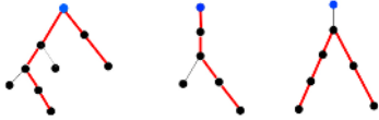
Fig. 3. Example of three situation of the longest path computation. blue vertex is the root node of tree, and red path is the longest path of tree.
