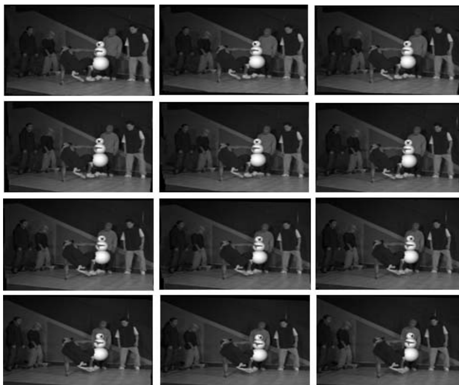
Fig. 7. Four base camera images (left column) and eight virtual images (middle and right columns) combined with a synthetic graphic object "snowman"
