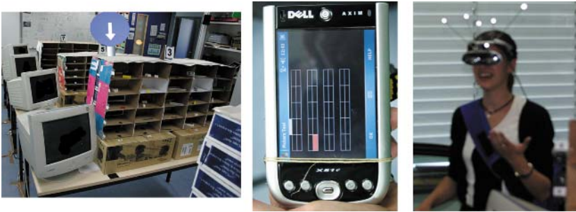
Fig. 2. Warehouse setup for the Wayfinding test with a) spatial b) hand-held and c) head-attached displays
