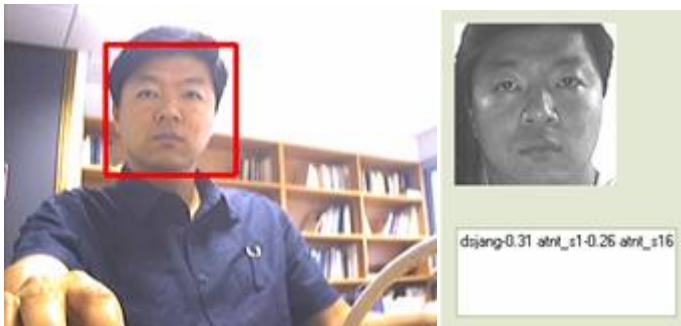
Fig. 8. Face recognition using an embedded HMM. It can detect a facial region (left) and recognize the face using face database. Actual output is converted to voice message and offered to the user.
