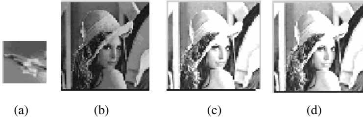
Fig. 1. (a) is the gray watermark that we would embed into the original image (b). After make DWT on original image (b), we get the LL sub-band image (c). Then embed the gray watermark (a) into the LL sub-band image (c). The result of the LL sub-band image after embed watermark. is (d).
