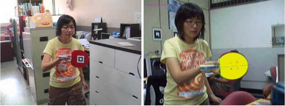
Fig. 6. The racket tracking by detecting the marker attached to the racket face
