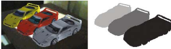
Fig. 3. Picking in the alpha channel, the RGB frame to the left and the corresponding alpha channel to the right
