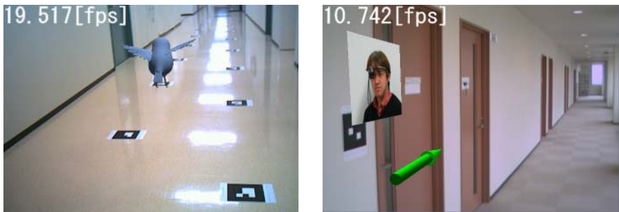
Fig. 4. The left figure is a screenshot of a Precision M60, which is implemented as an HLC. A fluttering bird guides the user to his/her destination. The right figure is a screenshot of VAIO Type U, which is implemented as an MLC. A user heading and an annotated image of a room are displayed.
