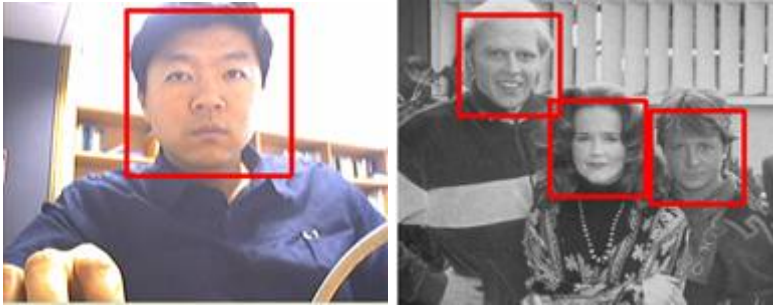
Fig. 5. An example of applying Haar face detection algorithm. Rectangles represent facial region on images.
