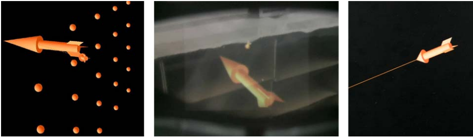
Fig. 5. Picking scenario. a) Arrow indicating the box to pick from and a ball in front of each box. b) The arrow seen through an HMD. c) Arrow with rubber band point at target.
