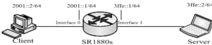
Fig. 8. Architecture of Testing Security Module with One Router
