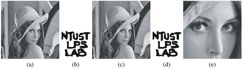
Fig. 3. (a) The test image “lena” of size 512 \times 512 , (b) the watermark, (c) the watermarked image obtained by our approach (PSNR=43.23), (d) the extracted watermark under no attacks (NC=1), and (e) the eyes part of watermarked Lena image obtained by proposed approach
