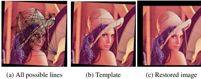
Fig. 3. After detecting peaks from ACF, all possible lines consisting 3 candidate peaks are selected like image (a). Lines are filtered by angle and distance conditions from all possible lines and construct a lattice-like template showed in (b). From the template reverse angle and scaling rates are calculated and restore image like (c).
