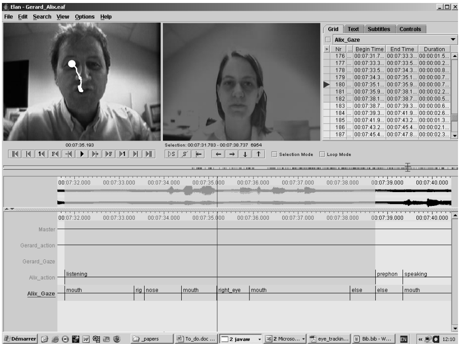
Fig. 5. Screenshot of the labeling framework for face-to-face interaction data (using the ELAN editor® www.mpi.nl/tools/elan.html ). The female listener fixates either the mouth or the right eye of the male speaker when he is uttering a SUS utterance (see text).
