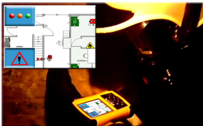
Fig. 1. The ruggedized PDA shows the floorplan and shows the status of the exploration
