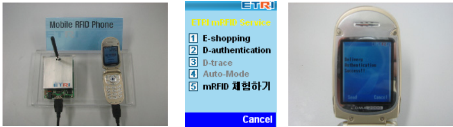
Fig. 6. Reference implementation of mobile RFID phone which provides information of a RFID tag to a mobile phone user
