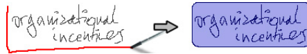
Fig. 6. Surrounding with a partial rectangle gesture creates a new node with the contained strokes as label
