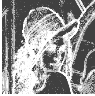
Fig. 5. The fitting function class in each image point is indicated: the higher (whiter) the point's intensity, the lower the node of the fitting function in the decision tree of Figure 3. When no correct approximation is found, points are colored white. The image was convolved first with a Gaussian of standard deviation \sqrt{2} .
