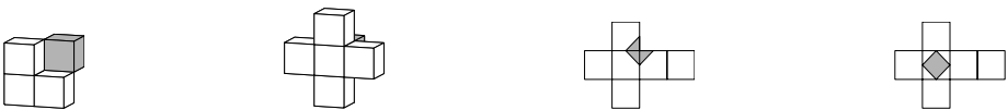
Fig. 4. Using these masks and the 7+5 symmetric masks for \mathbb{Z}^3 in Algorithm 1 will result in insufficient propagation of distances, e.g., for neighbourhood sequences with B = (1, 3)
