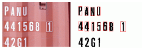
Fig. 3. Identifier area with a general color and successful results of edge extraction
