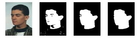
**Fig. 2.** Left to right: (a) Original image (b) Binary mask (BM) (c) Largest connected binary mask with holes filled (d) Binary mask after closing the gaps
