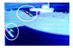
**Fig. 3.** Feature detection and tracking to estimate 2D camera egomotion. Red pixels are features detected in the current frame, green pixels are features detected in the previous frame (leftward motion shown). The motion of individual features is aggregated to determine global egomotion.
