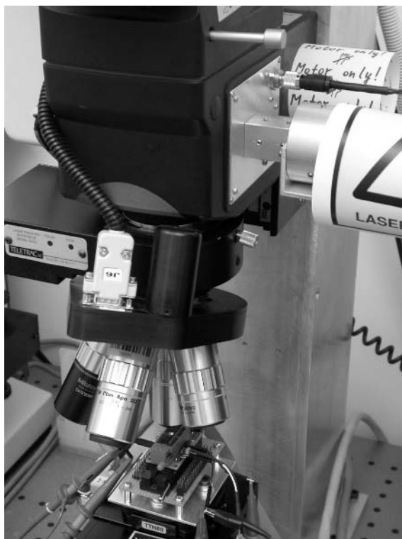
Fig. 2. Test setup for semi-invasive analysis
